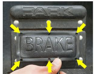
If mounting the switch using the Included Rivets, mark the hole locations and drill (6) 3/16" holes through the pedal. Mount the pad with the rivets.
