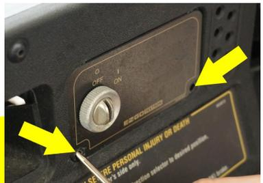
1. If powering the lights with the push-pull switch, disconnect the key switch. Using a vice or clamp to secure the plate, safely drill a 1/2" hole on the key switch plate. File any rough edges.
