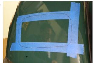
4. Using a jigsaw or rotary tool, cut out the INSIDE of the marked area. Test fit the taillight. If needed, make any modifications and retest. Once it is fitted properly, remove the tape and sand any rough edges.
