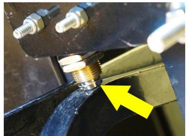
4. Slide the brake switch wire and the brake lead from the deluxe harness behind the bracket and down the channel with the existing harness.
