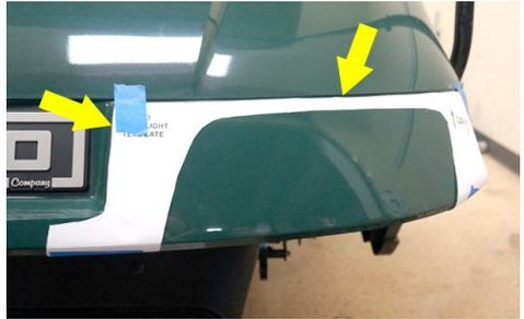
2. Using painter's tape, tape the template to the driver side front body of the cart. The dotted lines on the template will line up with the body lines of the cart.
