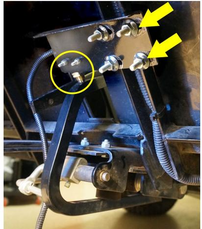
3. Position the bracket so the switch is centered above the pedal assembly. Lower it until the switch is activated (it will click). Tighten the nuts to lock the bracket into position.
