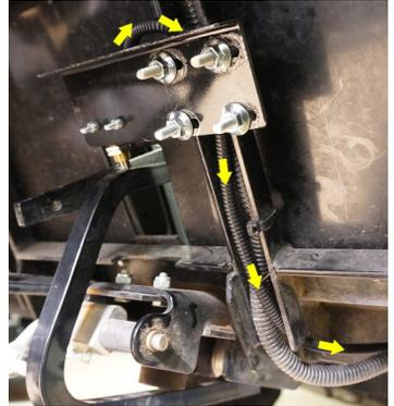
5. Install the LGT-142, time delay, near the first opening in the frame. Mark the hole location and drill an 1/8" pilot hole. Drill a 1/4" hole through the pilot hole. Mount the time delay with the Included Hardware.
