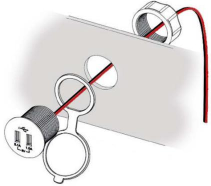
**NOTE:** A fuse holder (ACC-0019) and 15A fuse (ACC-0021) are recommended if direct connecting the USB ports to a 12V battery or voltage reducer.
