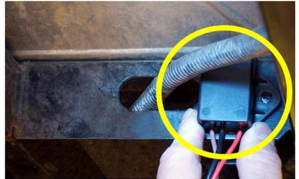
6. Connect the brake switch to the time delay and deluxe harness as shown in the diagram below.
