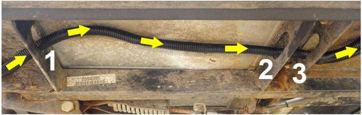
5. Route the taillight and battery connections through the access hole that leads to the battery compartment. Set the battery leads to the side. They will be connected after completing the installation of the harness, lights and/or accessories.
