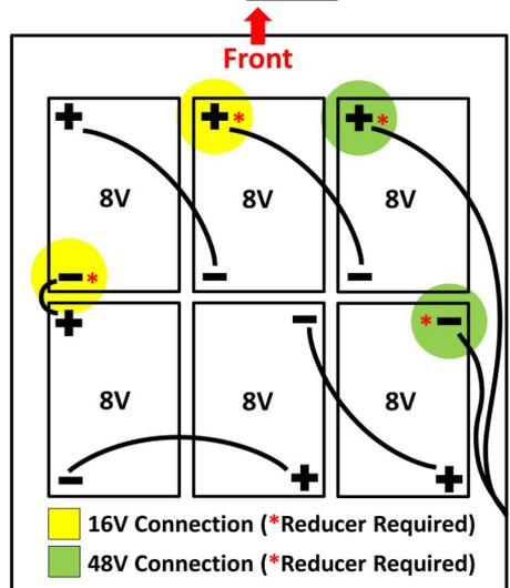
required to reduce the voltage to 12V. On a gas cart, connect the wires to the battery. Tighten the nuts but do not over tighten. Over tightening can destroy the battery posts.
