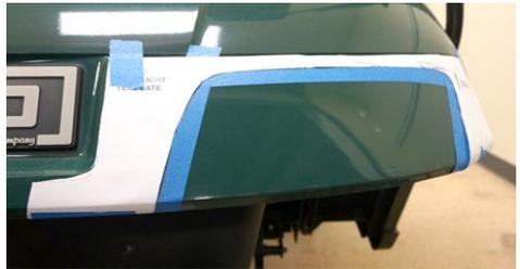
4. Using a jigsaw or rotary tool, cut the INSIDE of the marked area. Test fit the headlight. If needed, make any modifications and retest. Once it is fitted properly, remove the tape and sand any rough edges.
