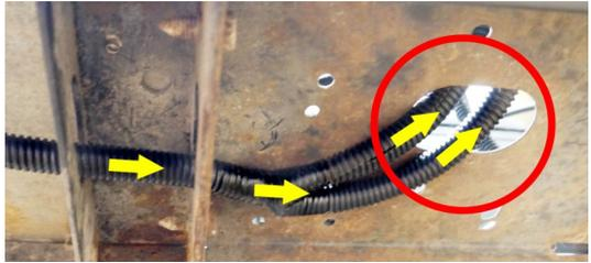
6. Route the taillight leads to the holes that were cut out for the taillights. The shorter lead will go over the driver side inner fender. The longer lead will go behind the battery pack and over the passenger fender.
