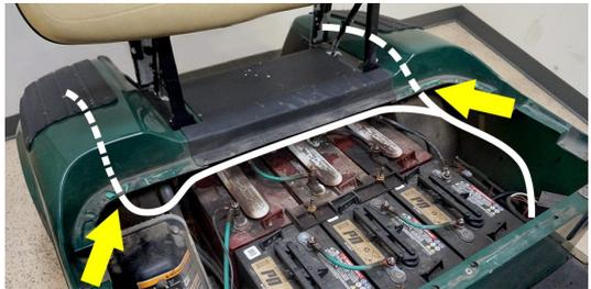
7. Route the front portion of the harness through the vertical channel on the driver side. Secure with cable ties.
