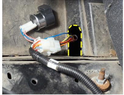
5. Access the connectors through the key switch plate. Connect the 9-pin connector on the turn signal switch to the 9-pin connector on the harness.
