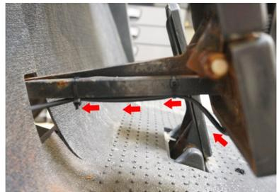
the assembly using cable ties.
