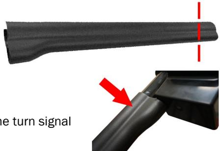
11. Snap the cover around the wires of the turn signal switch and the steering column.
